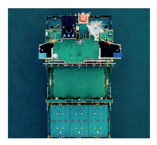
all manner of manufactured materials. Specially designed, fully cellular container ships carry containers stacked sometimes nine deep in the holds and four or five high on deck hatches. An increasing amount of cargo is carried on roll-on/roll-off ships, which are designed with large, clear vehicle decks to transport trucks and trailers.
